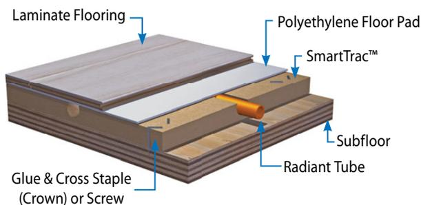
Prevent damage to laminate flooring by using controls that gradually adjust supply water temperatures with a reset curve. A floor temperature limiting sensor can be used to comply with flooring manufacturer's flooring temperature specifications.
