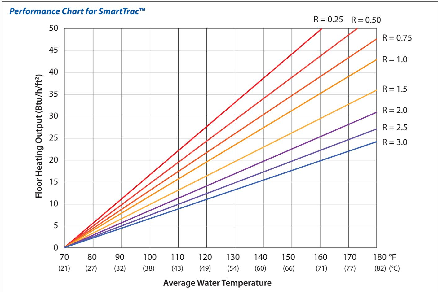
This chart shows average water temperature. In order to calculate required supply temperature, add half of expected delta-T to the average (i.e. add 10°F to the average if expected delta-T is 20°F). The performance above is based on typical construction practices and environmental conditions (at 70°F (21°C) room temperature). Actual results may vary.
