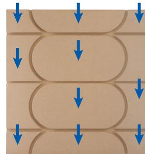
**When using staples instead of screws it is very important that the board is glued and stapled with the same quantity of glue and staple points as shown in the pattern above.** Cross stapling with a sheathing stapler is the fastest way to install SmartTrac™. 1-1/2" (38 mm) long, 16 gauge staples are recommended. Cross stapling means 2 staples are put closely together at opposing 45° angles. (45° angle to the surface)
