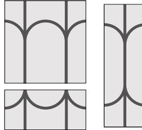
Various shapes can be cut from the Standard Panel to finish off areas of the room less than 24" (610 mm).
