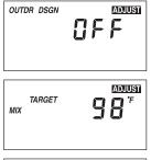
Press and release the *Item* button to advance to the OUTDR DSGN adjustment. Press and hold the A button until OFF is displayed.
