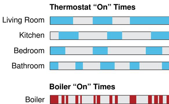
Without synchronization, the boiler is at the mercy of each zone. Non-communicating thermostats short cycle the boiler to achieve independent targets rather than system-wide goals. Boiler operation is inefficient & unreliable.
